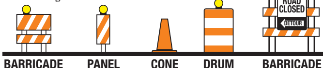
Channeling Devices used to direct traffic flow
